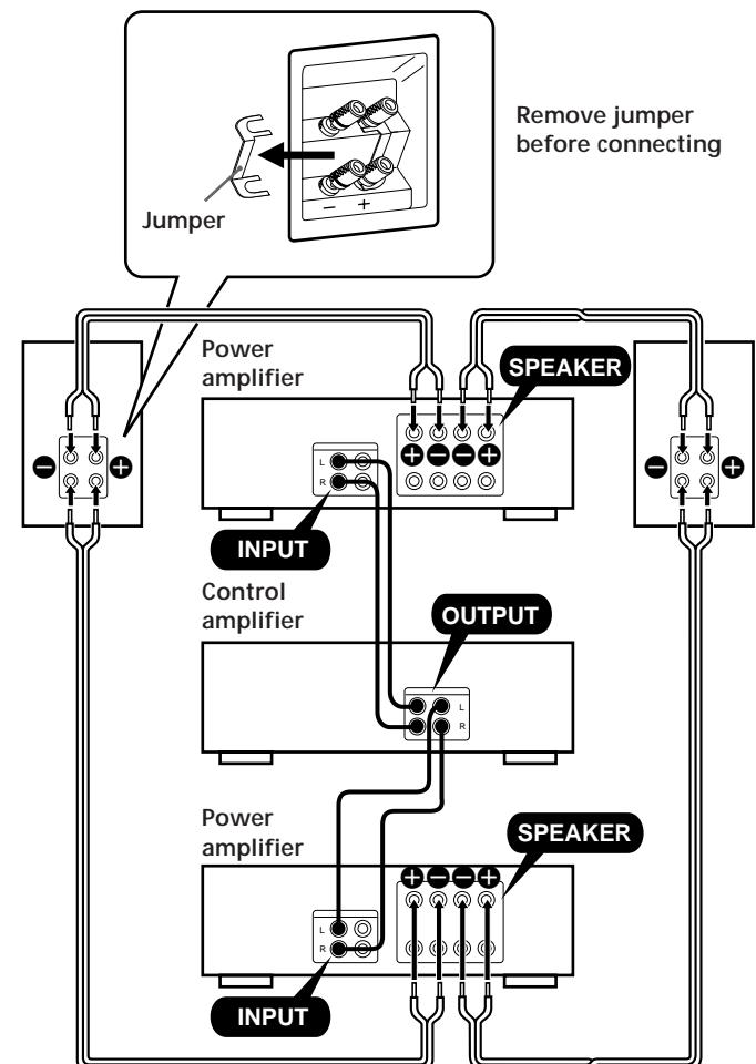
Connect the cord marked with a line (or lettering, etc.) to the "+" terminal
